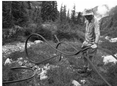
Snow-twisted rails near Mountain Lake Hut Photo: A. Purdey
